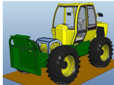
Fig. 7. Designed pedestal mounded on the rear part of the tractor frame
